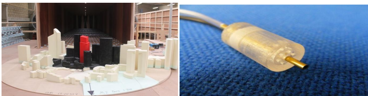
Figure 3.1 (a) Typical wind tunnel test setup. (b) Irwin probe sensors typically used to measure the pedestrian-level wind speeds.
